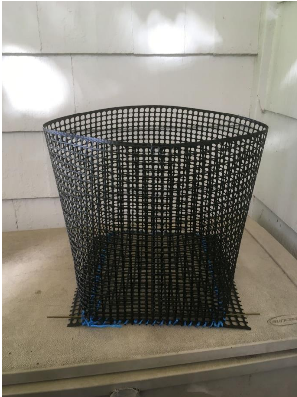
Ecoreactor 4, Photos 1 and 2: Shows a side and bottom view of E4. E4 differs from E3 in that all the sides of the ecoreactor are stitched with plastic string. In E3 most of the sides and bottom were stabilized to a wood frame. Either version works. The two variations were shown here for illustration purposes.
