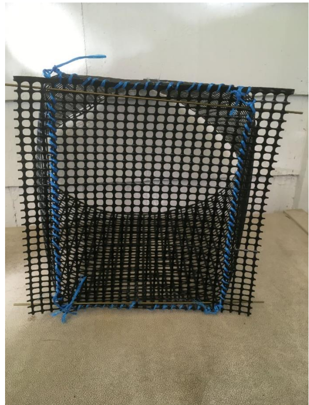
Ecoreactor 4, Photos 1 and 2: Shows a side and bottom view of E4. E4 differs from E3 in that all the sides of the ecoreactor are stitched with plastic string. In E3 most of the sides and bottom were stabilized to a wood frame. Either version works. The two variations were shown here for illustration purposes.
