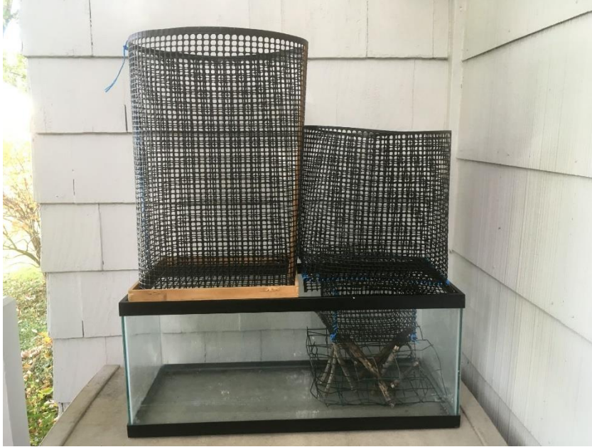
Photo 4: Shows an alternative placement of the four ecoreactors in the 20 gallon aquarium where a smaller E4 is placed above E2.
