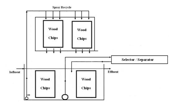
Here is a diagram is looking straight down at the tank with submerged chip baskets.
