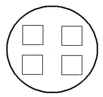
Each of the submerged and irrigated small chip baskets will have a volume of 63 gallons and will hold wood chips at a density of 2 pounds per gallon. Thus there will be a total of 504 pounds of wood chips in both the submerged and irrigated baskets for a total wood chip loading of 1,008 pounds, dry weight.
