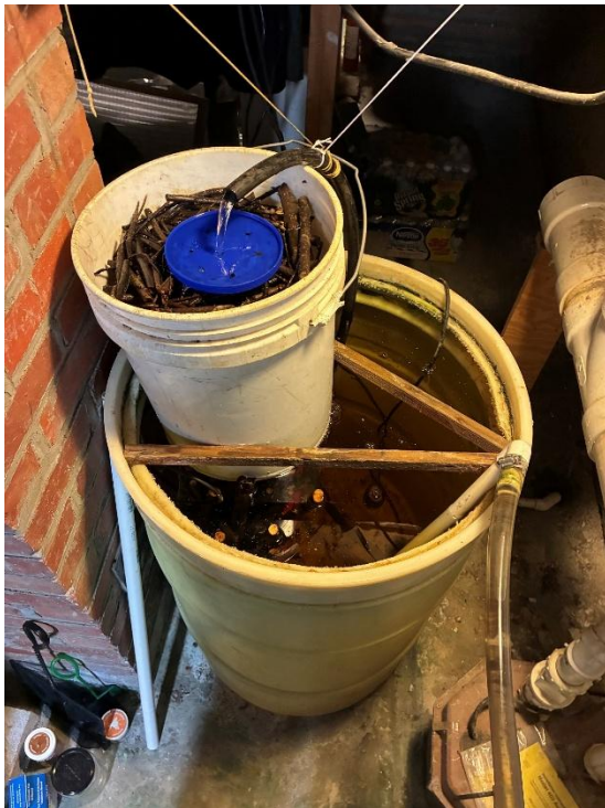
Added more sticks to a 5 gallon pail with holes in the bottom and put it on top of the sticks in the milk crate.
