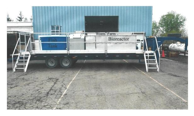
The system includes blowers, pumps, sensors, level controls, an electrical panel, process control instrumentation, phase converter if necessary, and internet connectivity. The trailer deck is 30 inches above ground level. It has
