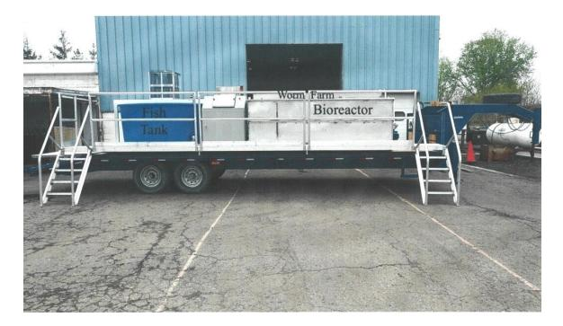
The system includes blowers, pumps, sensors, level controls, an electrical panel, process control instrumentation, phase converter if necessary, and internet connectivity. The trailer deck is 30 inches above ground level. It has
